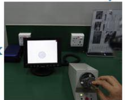
Cleaning end face
