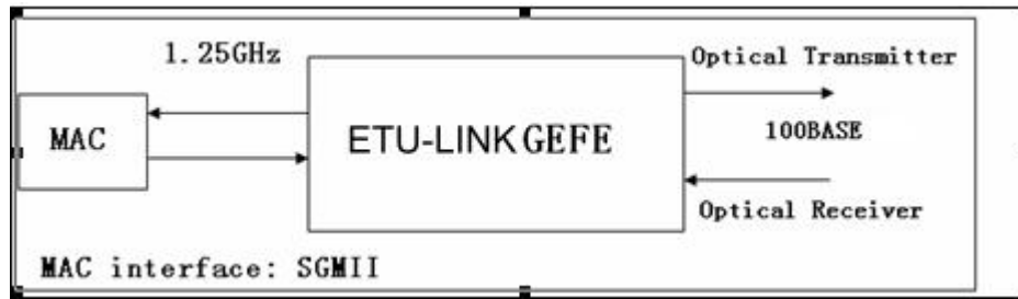
Figure 1. MAC to Fiber Connection
