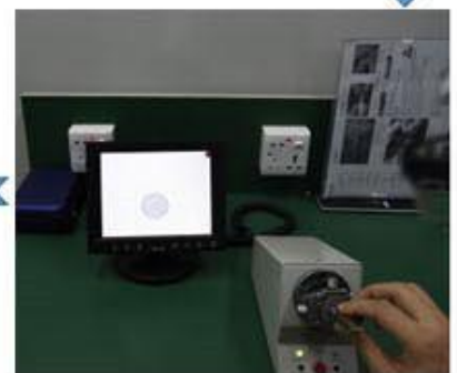
Cleaning end face
